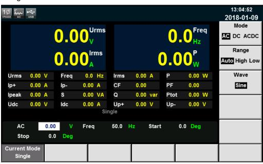
AC: AC voltage value. Setting range is different among Auto, High and Low range. Refer to 9.1 Main technical parameters for more details.
