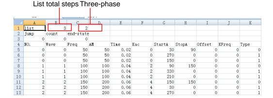
During the editing of the CSV files, corresponding waveform codes are as shown in the table below. The triggering types of List file are TIME and TRIG. TIME is represented by 0, TRIG 1.
