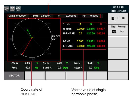
Coordinate of maximum value: display the maximum U, I or UI values of the phases A, B and C.
