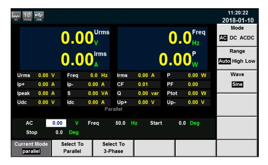
Press [Select To 3-Phase] to enter the three-phase function configuration interface. Press [Enter] to confirm. The master interface shows as follows and the slave interface displays PHASE B and PHASE C. This means the 3-phase parallel configuration is successful.
