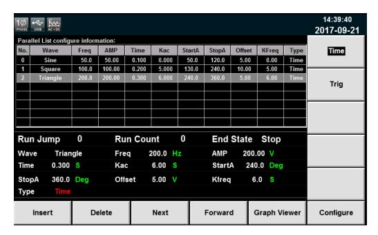
5. Press [Graph Viewer] to draw the waveform according to the configured parameters, as shown in the figure below.
