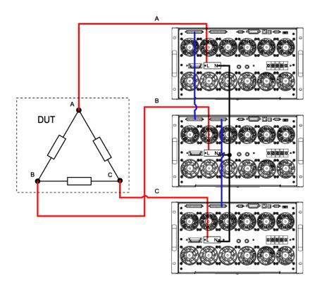
The system bus interface can be connected to multiple units via cross-over cables, as shown in the above connection of diagram of three-phase parallel power supplies. Select one connection method as shown above. After wiring, configure relevant parameters of the functions of the three-phase AC power supply.
