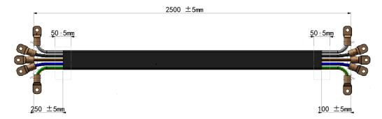
Connect the five terminals brown to line (L1), gray to line (L2), black to line (L3), blue to neutral (N), and yellow-green to ground (PE) on the other end of the power cord to your AC distribution panel.
