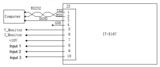
When using the RS-232 interface for communication, connect the pin 1, pin 2, and pin 3 of the IT-E167 to the PC. The pin description is as follows:
