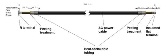
The yellow-green wire is grounding wire, which is connected to the PE terminal of power input on the rear panel; the others are live wires, which are correspondingly connected to the L1, L2 and L3 terminals of power input on the rear panel of the instrument.
