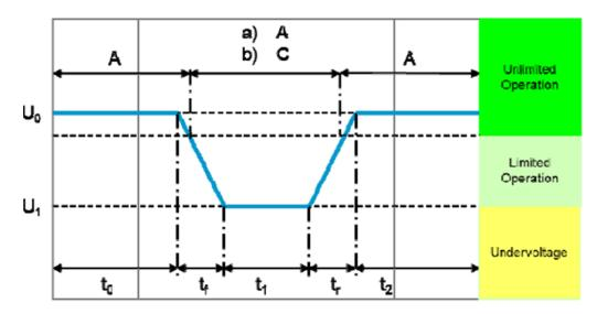
₣Test pulse parameters for E48-10 Starting pulses
