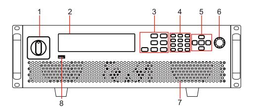
1 Power On/Off switch 5 Up, down, left, and right cursor navigation
