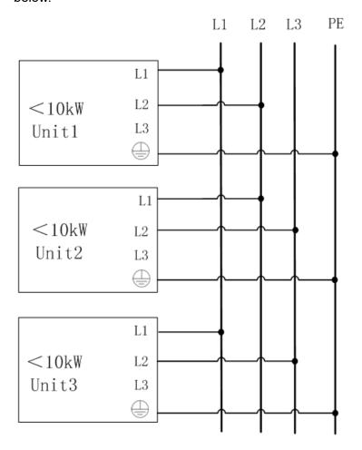
When connecting the instrument which rated power with 10kW≤ Power <
