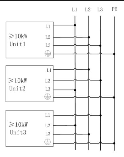
• The instrument which rated power great than or equal to 15kW, they already consume balanced current on all three phases. connecting the power cord as below.
