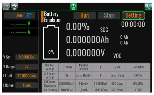
Click **[Setting]** to enter the battery simulation editing interface, and the parameters are described below.
