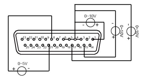
When 0V is input, the instrument's On/Off state is switched to Off state. When 5V is input, the instrument's On/Off state is switched to On state.
