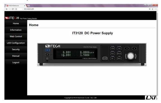
You can select different interfaces by clicking the seven buttons shown in the navigation bar on the left side of the window. The detailed descriptions are as follows.
