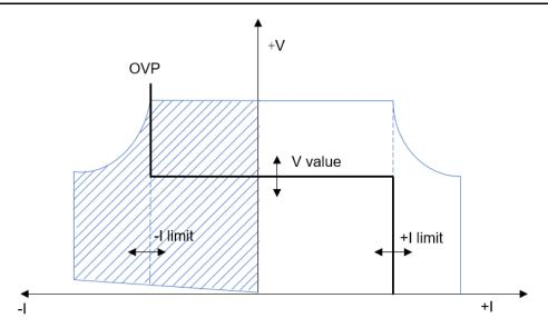
The heavy solid line illustrates the locus of possible operating points as a function of output. As shown by the horizontal portion of the line, the output voltage remains regulated at its programmed setting as long as the load current remains within the positive or negative current limit setting. A CV status flag indicates that the output voltage is being regulated and the output current is within its limit settings.
