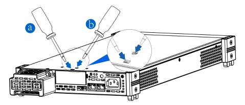
2. Install the purchased communication card. Taking the LAN+USB interface card as an example, push the card into the slot and secure with the screws
