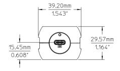
Figure 5. Mechanical dimension of U1832A
