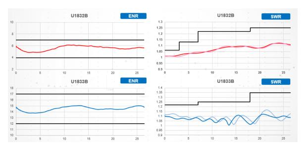
Figure 3. Typical ENR and return loss of U1832C and U1833C
