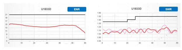
Figure 4. Typical ENR and return loss of U1833D
