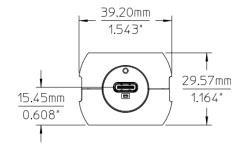
Figure 6. Mechanical dimension of U1832B
