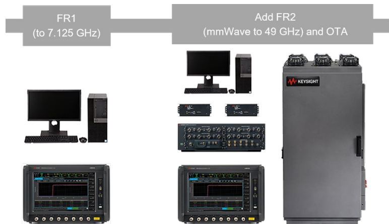
Figure 21. 5G NR FR2 mmWave test configuration
