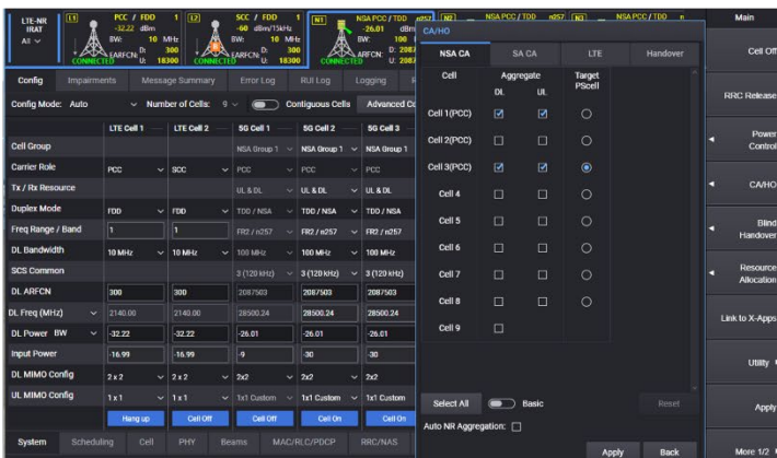
Figure 10. Handover test configuration
