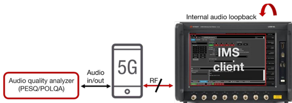
Figure 13. IMS test configuration for voice and video
