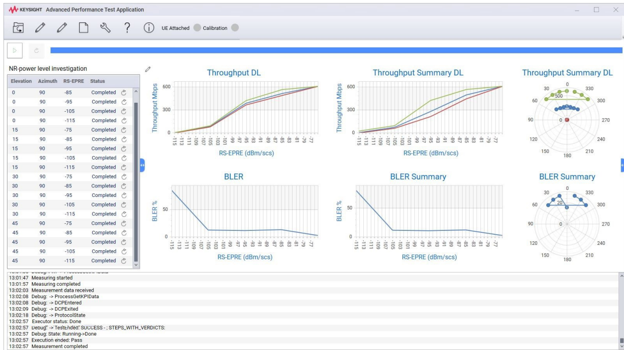
Figure 4. Test execution view from the S8708A Advanced Performance Test software in mmWave MIMO OTA view.
