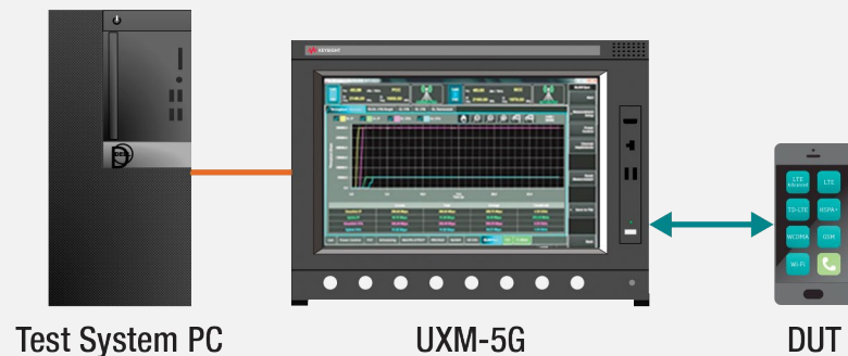
Figure 12. Test setup for sub-6GHz in Standalone or Non-Standalone mode.
