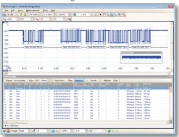
The PicoScope 6000 Series oscilloscopes are well-suited to serial decoding, with a deep memory buffer that allows them to collect long, uninterrupted sequences of data. This allows the capture of thousands of frames or packets of data over several seconds. The scopes can decode up to four buses simultaneously with independent protocol selection for each input channel.
