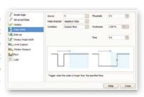
All triggering is digital, resulting in high threshold resolution with programmable hysteresis and optimal waveform stability.
