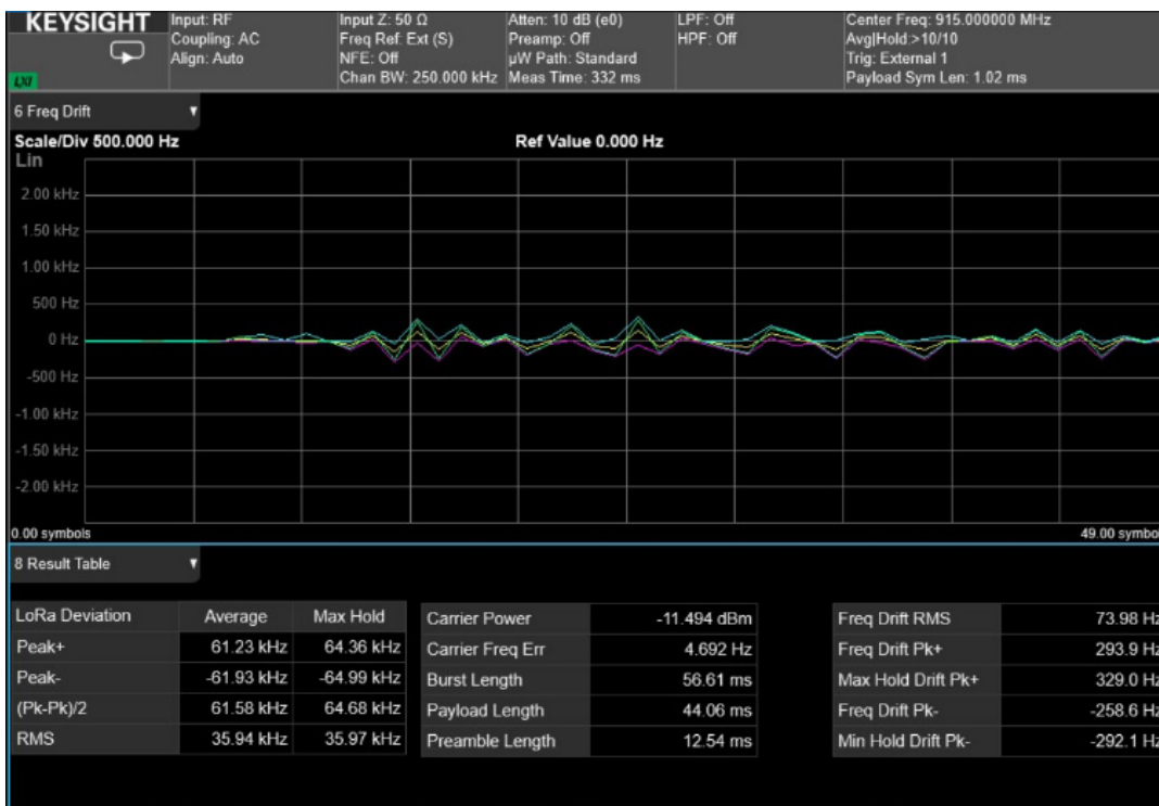
Figure 6. LoRa® modulation analysis Frequency Drift
