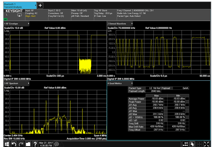
Figure 4. Transmit analysis for low energy (LE) signal
