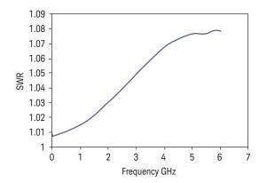
Typical SWR, 100 kHz to 6 GHz (25 ±10°C) for N8482H power sensor
