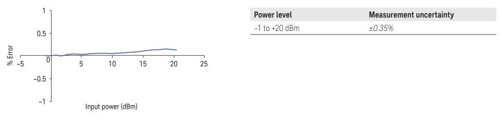
Typical N8481A/2A/5A/7A/8A and N8486AR/AQ power linearity at 25°C, after zero and calibration with associated measurement uncertainty
