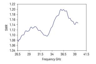
Typical SWR, 26.5 to 40 GHz (25 ±10°C) for N8486AR power sensor
