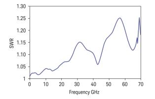
Typical SWR, 10 MHz to 70 GHz (25 ±10°C) for N8488A power sensor
