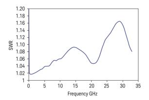
Typical SWR, 10 MHz to 26.5 GHz (25 ±10°C) for N8485A sensor
