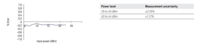
Typical N8481B/2B power linearity at 25°C, after zero and calibration with associated measurement uncertainty
