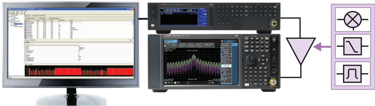
Figure 1. Typical component test configuration using Signal Studio's basic capabilities with a Keysight X-Series signal generator and an X-Series signal analyzer
