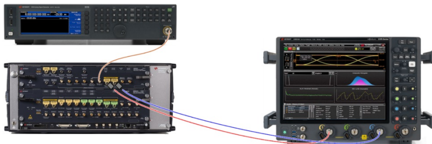
Figure 3: Stress signal calibration at TP3' or Case 1 with pattern generator and common-mode interference source
