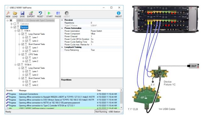
Figure 3: Receiver Tests and long channel receiver test setup
