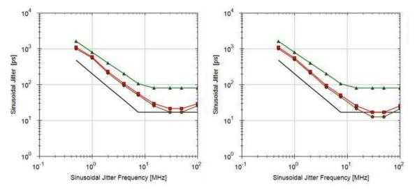
Figure 4: Jitter tolerance test result of a USB 3.2 product operating in single lane mode (left) vs dual lane mode (right)
