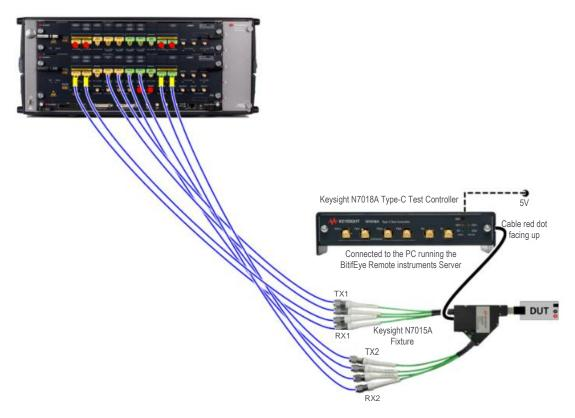
Figure 6: Receiver test setup with N7015A and N7018A
