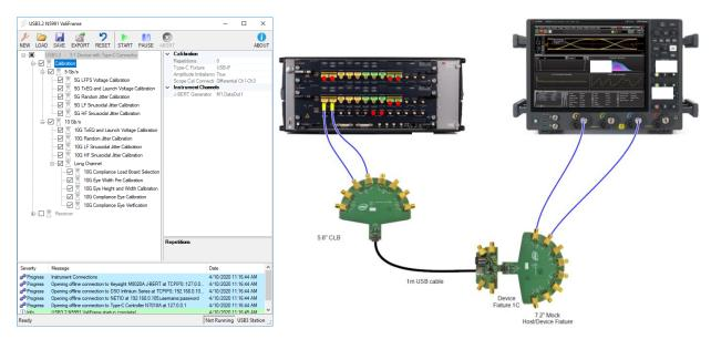
Figure 2: Receiver Calibrations and 10 Gb/s long channel calibration setup
