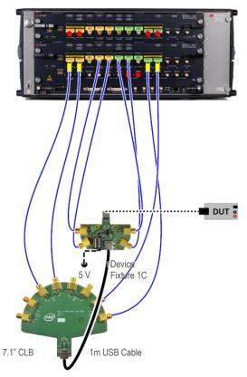
Figure 5: Dual lane receiver tests and long channel test setup
