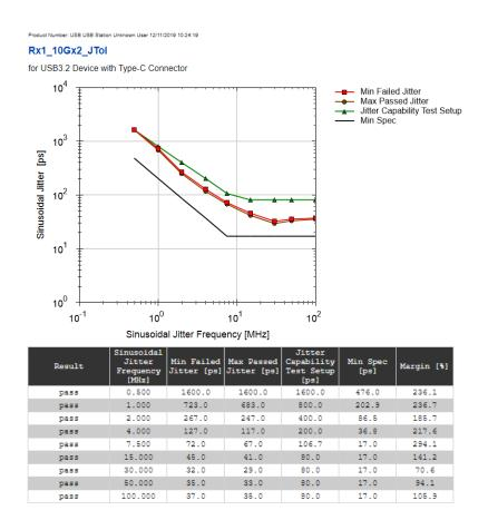
Figure 1: 10 Gb/s dual lane jitter tolerance test result
