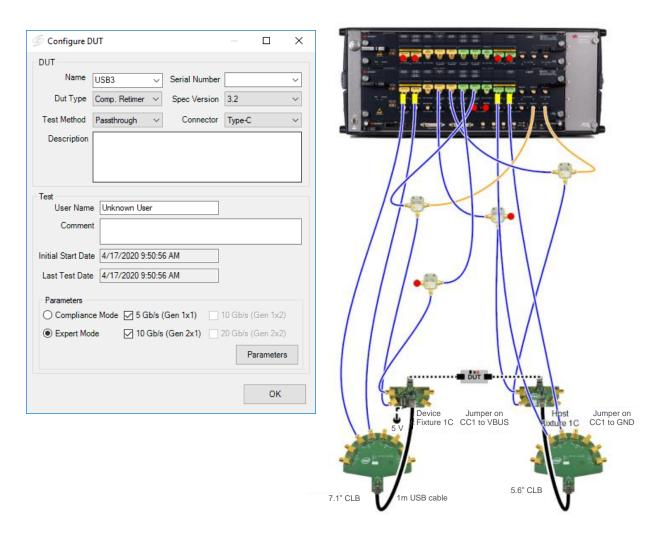
Figure 7: Component retimer configuration and receiver test setup in passthrough mode
