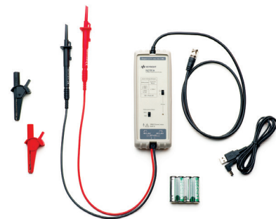
N2791A 25-MHz, 700-V differential probe
