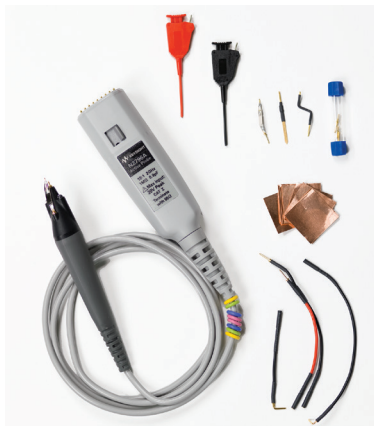
N2795A/96A active probe with standard accessories
