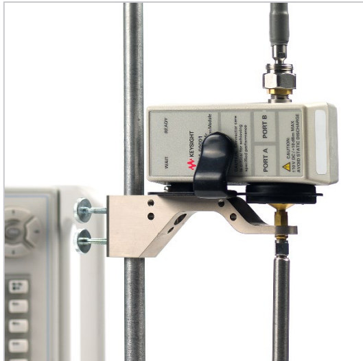
Figure 13. ECal module connected in line for electronic
