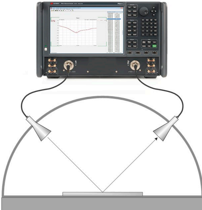
Figure 7. In the NRL arch method, one antenna transmits energy onto the MUT and the second antenna receives the reflected portion.
