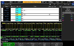
Figure 15. I2C decode and trigger.
