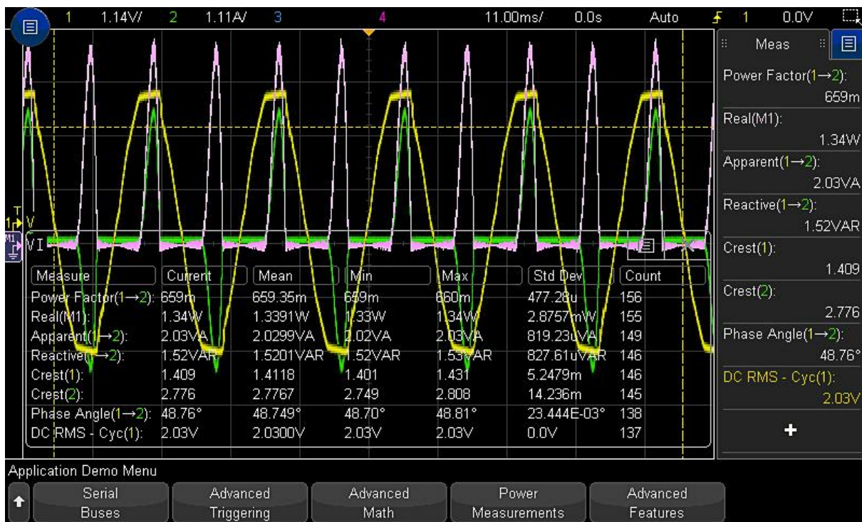
Figure 28a. Integrated power measurements make quick work of analyzing power producing and power consuming devices.
