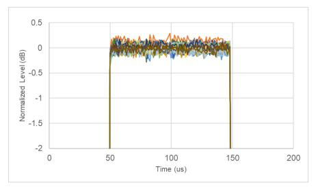
1. Measured with a 500 kHz IF bandwidth, no averaging (Average Type = Point). With 100 us pulse width setting. 50 us/div.
