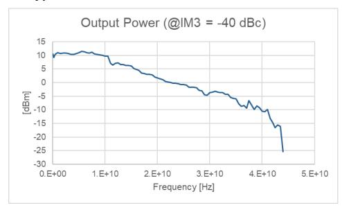
1. Measured tone power at test port 1 with -40 dBc IM3 with two-tone signals. 1 MHz tone separation, 0 dB source mixer attenuator.
