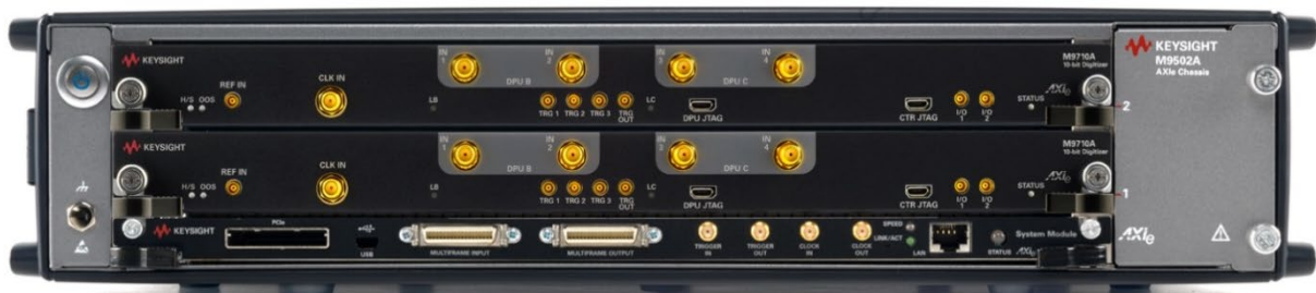
Figure 2. Two M9710A digitizers installed in the M9502A 2-slot chassis, forming an 8-ch 10-bit acquisition system.
