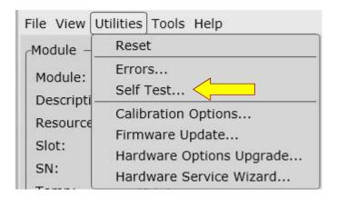
The Self-Test Dialog Box will appear. Click "Run Self Test" to start a self-test.
