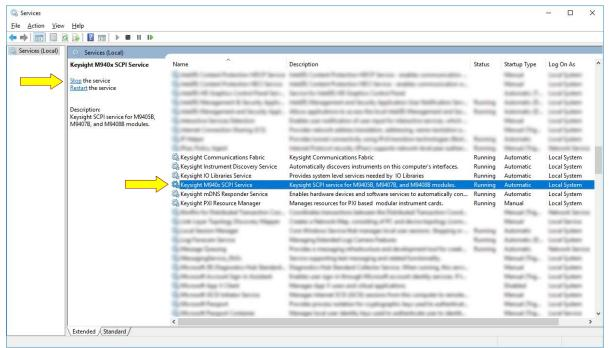
To prevent the SCPI service from starting automatically, right click on "Keysight M940x SCPI Service" and select "Properties". From the properties window select "Manual" from the "Startup type" drop down menu and click "OK" (Figure 10).
