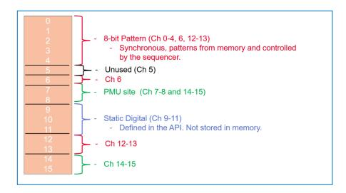
Digital channel direction and timing can be flexibly controlled on a per digital vector basis. The cyclized data allows each pin to operate in RZ or NRZ modes. In combination with the 1 ns edge placement resolution, each pin allows for an adjustable output delay, for timing margin testing, and receive delay to compensate for cabling propagation delays.
