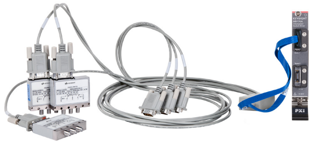
Figure 3. Drive three SPDTs with M9170A using Option 601 interface cable
