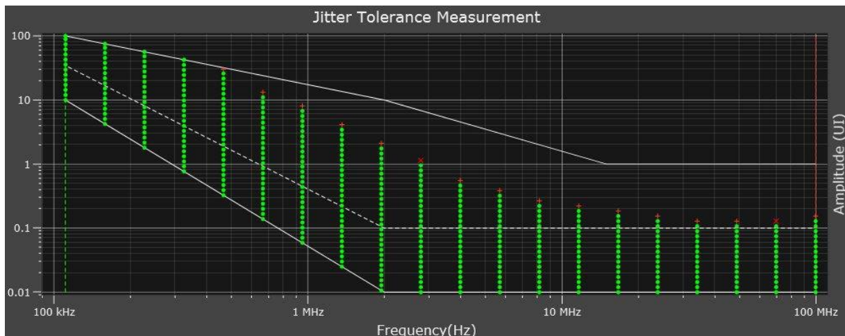
Figure 6. J-BERT M8020A provides automated jitter tolerance characterization and compliance measurements. A library of Jitter tolerance templates is available. To optimize test time, customized jitter tolerance templates can be created with a graphical jitter tolerance template editor. The red dots in the result screen show where the BER level was exceeded, the green dots show where the DUT tolerated the received jitter.
