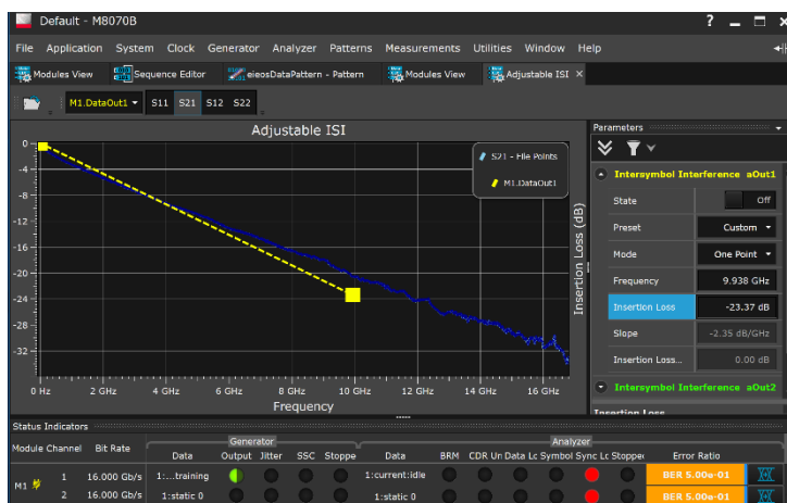
Figure 8. J-BERT M8020A offers integrated and adjustable ISI to emulate channel loss. ISI can be controlled for each channel independently via a graphical user interface. Frequency and loss points can be set. S-parameter files can be imported. The example shows a loss curve in blue for the imported S21 parameters for the 12.8 "trace of M8048A. The red line shows the loss parameter entry for M8020A.
