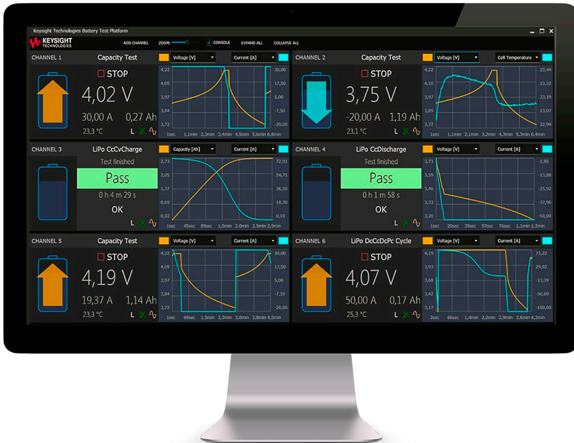
Figure 5. TAP's API enables user-developed GUIs that help operators easily visualize test results.
