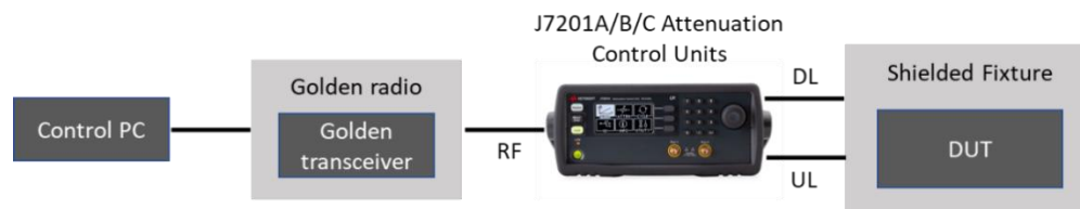
Figure 1. Simplified test setup for mobile receiver sensitivity test using a golden radio
