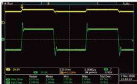
Control loop CV priority mode
