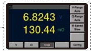
High speed simultaneous resistance and voltage measurement.
