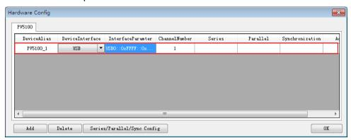
To change default parameter of hardware device (e.g., device interface, interface parameter and channel number), you may click the parameter for change.
