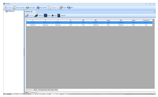
In the check interface of statistics information, the user can also select the Excel/Voltage Wave/Resistance Wave tab for detailed check of measurement data information.
