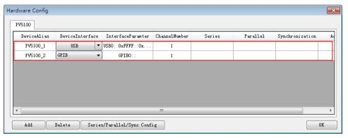
Click "Series/Parallel/Synchronization" button and click "Synchronization" in the figure below.
