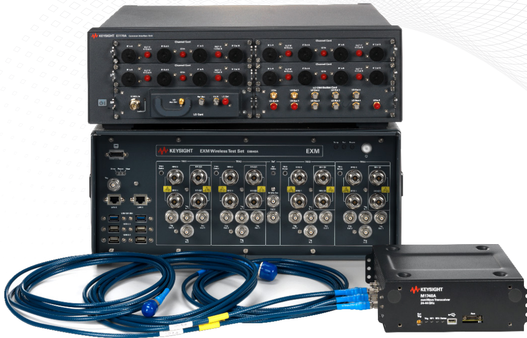
Figure 1: EXM mmWave configuration with E7770A and M1740A
