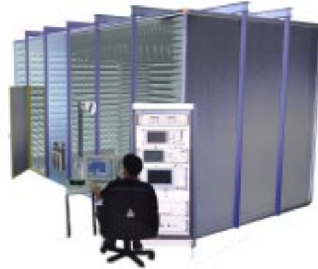
ETS-Lindgren Antenna Test Lab with Optional Test Instrumentation
