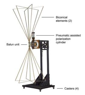
The pedestal allows antenna height and tilt-angle to be easily adjusted, plus features a wheeled base so that the antenna can be rolled out of the chamber and stored when not in use. Slots below the base allow for easy transport with a pallet jack or forklift. Horizontal and vertical polarization rotation is performed by a toggle switch on the back. The air valve assembly for pneumatic polarization is mounted onto the mast.
