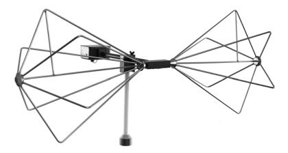
The biconical elements are made from welded aluminum. The elements mount in a balun network fabricated of phenolic and equipped with the necessary impedance-matching components. The lightweight construction provides easy handling and storage.
