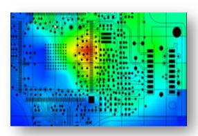
EMC and signal integrity are major concerns in the design of ultra-high speed (>2 GHz) PCBs. EMScanner enables the design engineers to diagnose EMC/EMI problems between 150 kHz and 8 GHz.
