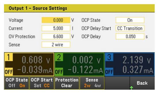
Figure 1. On E36312A or E36313A set 2-wire or 4-wire sensing for output 1 in just one click
