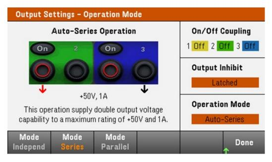
Figure 2. Auto-series operation to double the output voltage
