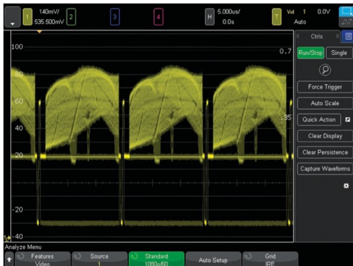
Figure 27. Triggering on 1080p HDTV signal analysis.
