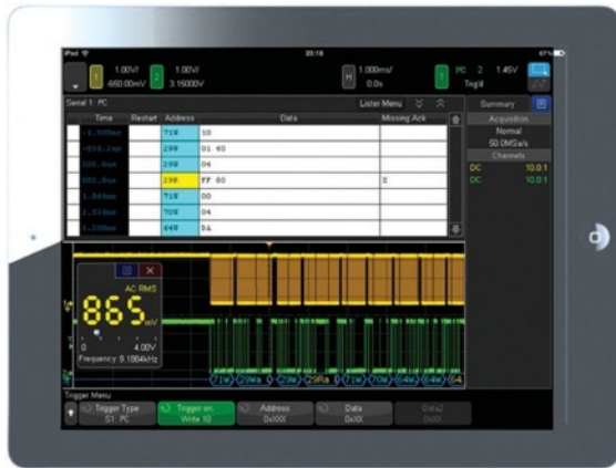
Figure 37. Tablet virtual front panel control.
