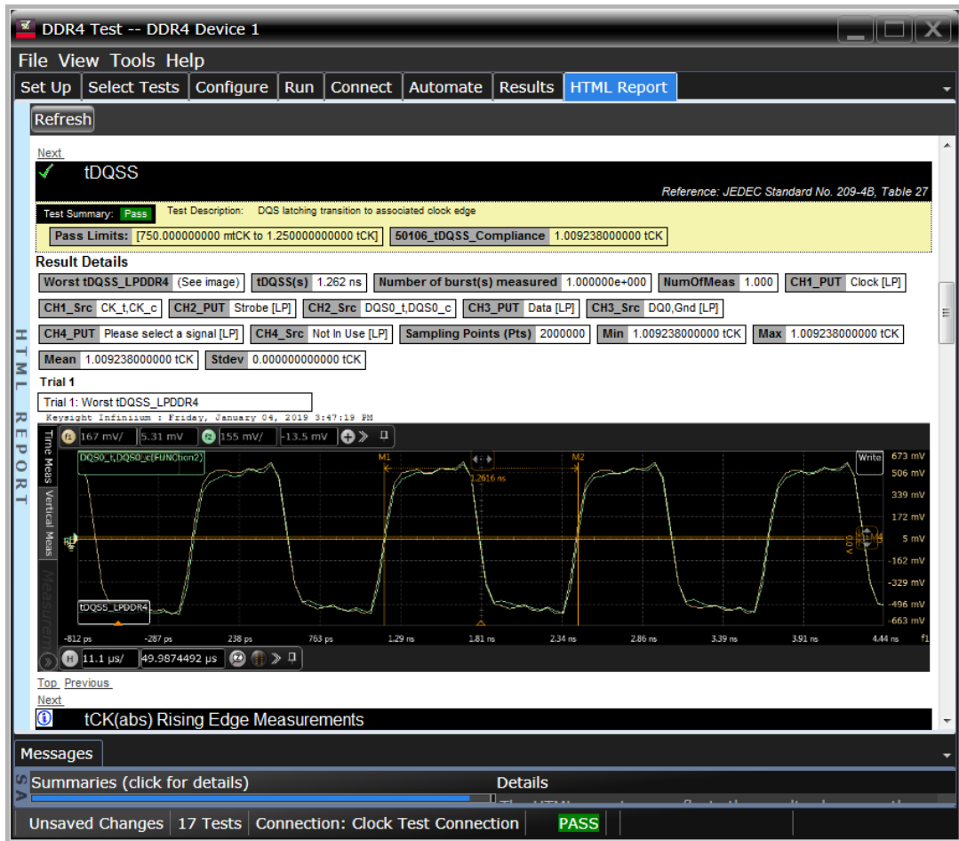
Figure 6: The DDR4 and LPDDR4 test application generates a summary report for quick results viewing. The report includes details such as test limits, test description and test results.
