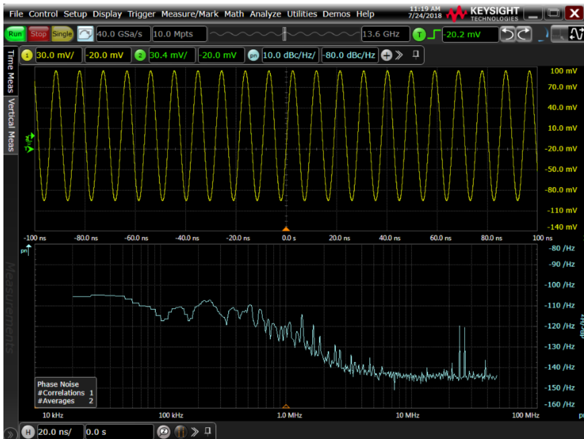
Figure 8. Using default settings, spurs in the spectrum are normalized into the plot.
