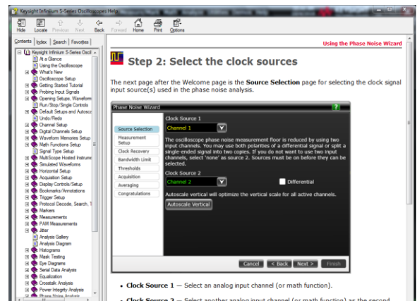
Figure 4. Infiniium built-in help guides walk you through automatic wizards, as well as manual step-by-step setup of all jitter and phase noise measurements.
