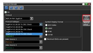
Figure 1. Set up your scope to show any protocol decode in seconds using the Auto Setup key.
