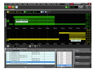
Figure 2. Time correlation between signal and decoded data.
