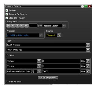
Figure 3: Fully customizable protocol searching and triggering.
