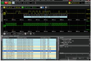
Figure A dual view showing the physical layer with a time-aligned decode, as well as a smaller protocol table below.
