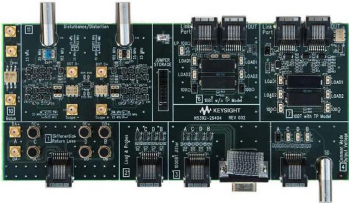
Figure 7. The N5395C standard Ethernet test fixture allows you to test the 10BASE-T, 100BASE-TX and 1000BASE-T transmitter signals. The fixture kit includes a CAT5E cable and the return loss fixture shown below.
