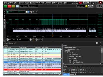
software-based triggering or hardware-based serial triggering. With protocol triggering, the oscilloscope takes signals acquired using either a scope or digital channels and reconstructs protocol frames after each acquisition. It then inspects these protocol frames against specified protocol-level trigger conditions and triggers when the condition is met.
