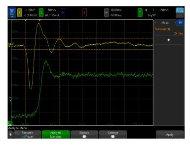
Figure 8. Transient response settling time measurement.
