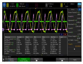
Figure 1. Input AC power quality measurements.
