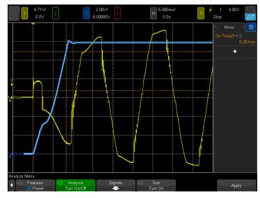
Figure 7. AC-to-DC turn-on time measurement.
