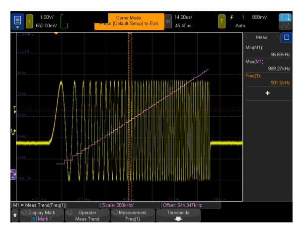
Figure 16. Measurement trend math function used to plot frequency versus time of a FM burst.
