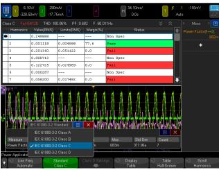
Figure 2. Current harmonics measurement based on IEC 61000-3-2 standards.
