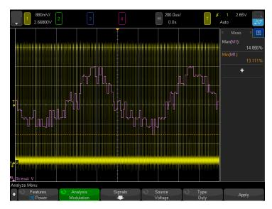
Figure 5. PWM duty cycle versus time.
