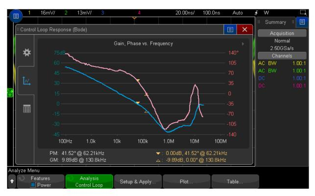
Figure 10. Control loop response gain & phase measurement.
