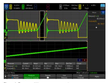
Figure 4.  $R_{DS(ON)}$  and  $V_{CE(SAT)}$  measurements.
