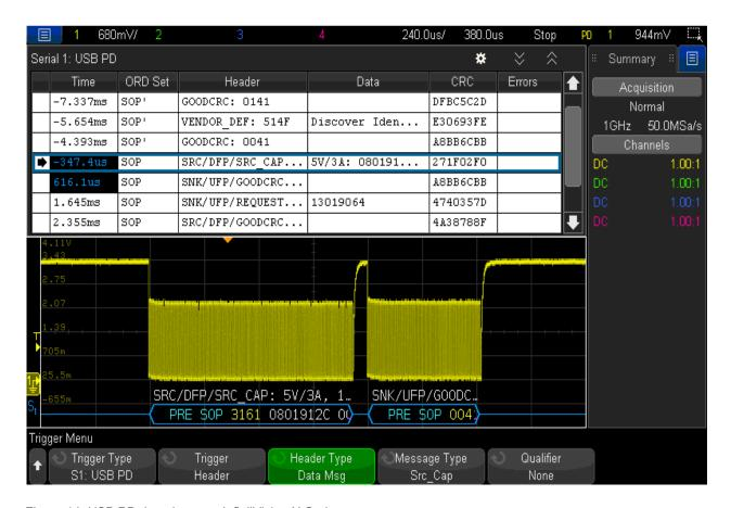
Figure 14. USB PD decode on an InfiniiVision X-Series
