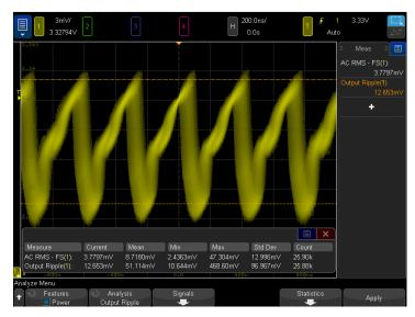
Figure 6. DC-to-DC converter output ripple measurement.
