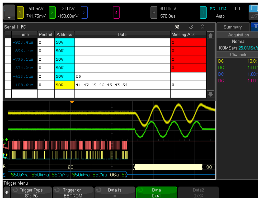
Figure 1. Decoding and triggering on an I 2 C bus using a Keysight mixed signal oscilloscope (MSO) licensed with the Embedded Software Package.
