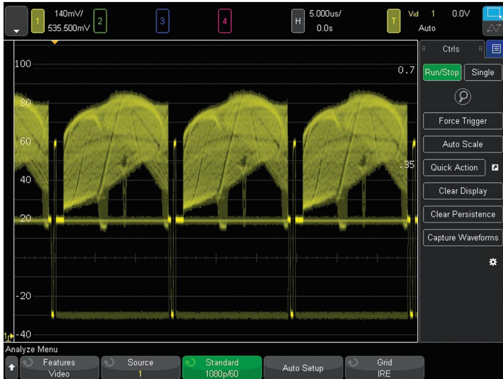
Figure 9. Triggering on 1080p HDTV.
