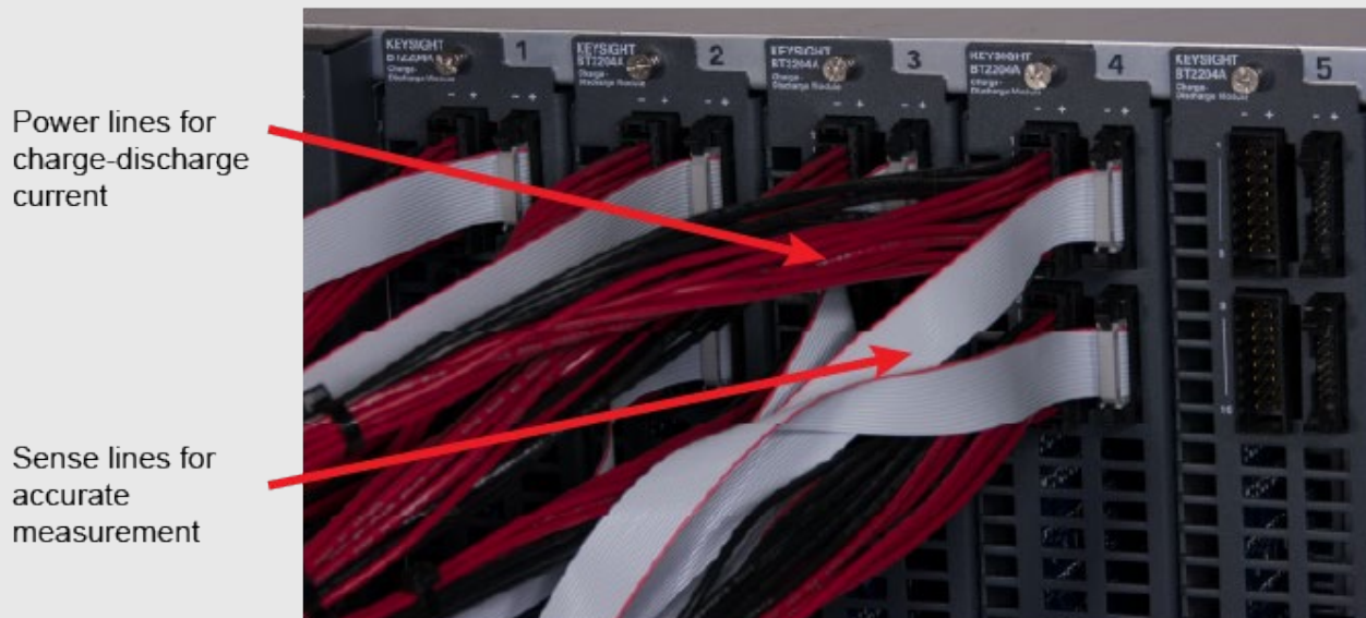
Figure 4. 4-wire connections (power and sense) to cells enable accurate measurements even with long cables to your fixture
