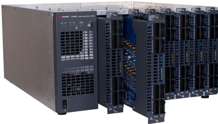
Figure 1. BT2203B chassis with 8 BT2204B modules
