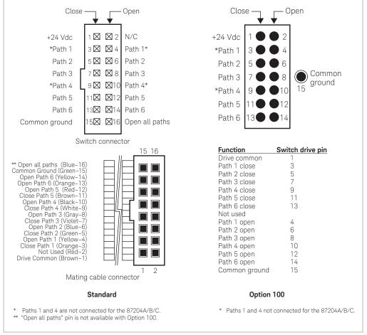
Figure 8. Drive connection diagrams
