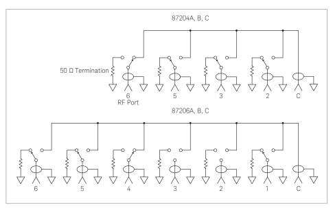
Figure 1. Keysight 87204A/B/C and 87206A/B/C simplified schematics
